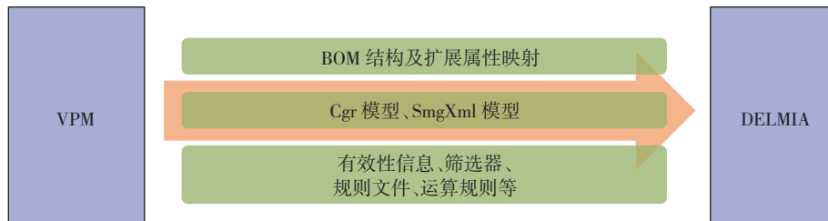
图5 VPM与DELMIA数据传递 Fig.5 VPM and DELMIA data transfer
